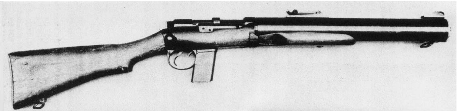
DeLisle .45 ACP Commando Carbine with integral suppressor
